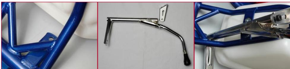
**THE SEQUENCE OF THE MODIFICATIONS TO SWITCH FROM A KF TO A KZ** Above, to the left, the KF chassis with the hooks that "transform" it into a chassis for geared karts. Centre, the shift lever and, to the right, the fixture assembled on the body frame. Below, the Chiesa Corse kart.
